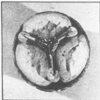
Cut open view of used DISPOSABLE steam cylinder with rock hard mineral deposits after 1-1/2 years of operation.
